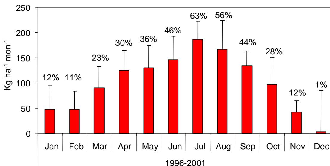
**Figure 2.** Seasonal variation in area specific and relative tot-N removal in the FWS wetland Magle receiving biological and chemically pretreated wastewater from Hässleholm municipal wastewater treatment plant. Error bars denote std error. (From Andersson & Kallner Bastviken, 2002).
