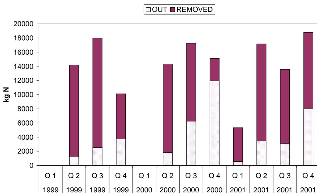
**Figure 3.** Quarterly load, removal and outflow of tot-N at wetland Alhagen, Nynäshamn, receiving chemically treated municipal wastewater. Total area of the wetland system is 28 ha. The data for quarter 1 in 2001 are from March only.
